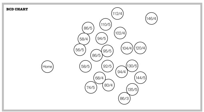
NOTE: Place center of drive side crankarm over "home", and pivot crankarm until chainring hole lines up with numbered outer circle.
