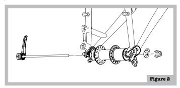
3. Reinstall wheel and tighten QR axle to manufacturer's specification.
