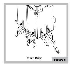
2. Secure Velcro straps around the rack platform tubes and back on to the bag, securing the bag to your rack (Figure 4). Use the roll-top closure straps as extra security by passing the buckles around the rack tubes before buckling the roll-top closure.
